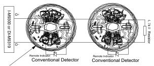
DO NOT USE LOOPED WIRE UNDER TERMINAL 3, BREAK WIRE RUN TO PROVIDE SUPERVISION OF CONNECTIONS
